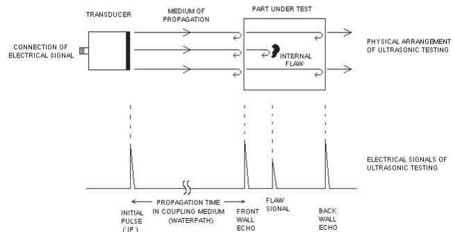
Basic principle of ultrasonic testing by "pulse-echo" method.
